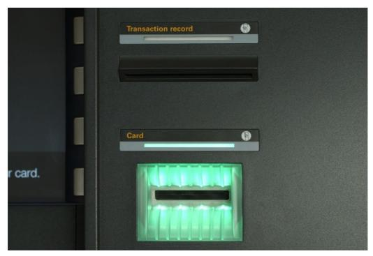
Figure 6. The receipt slot and, below it, the ridged card slot.
