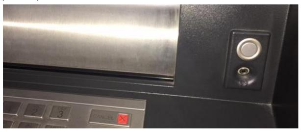
Figure 2. The audio input jack is located above and to the right of the keypad.
